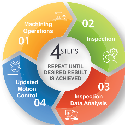
Figure 3. The process of continuously measuring outcomes of a machining operation with non-contact CMM technology to continuously adjust for the difference between the actual and desired geometric machining results.
